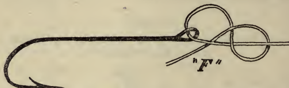
Fig. F:—This is another method, a bit more complicated. The knot is first tied as above, then slipped over the eye and drawn tight.
