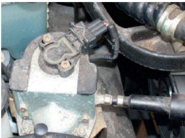
Figure 3.110 Throttle motor connected to cable
