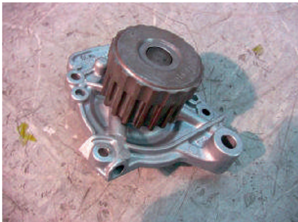
Figure 2.165 Water pump drive gear (cam belt)
