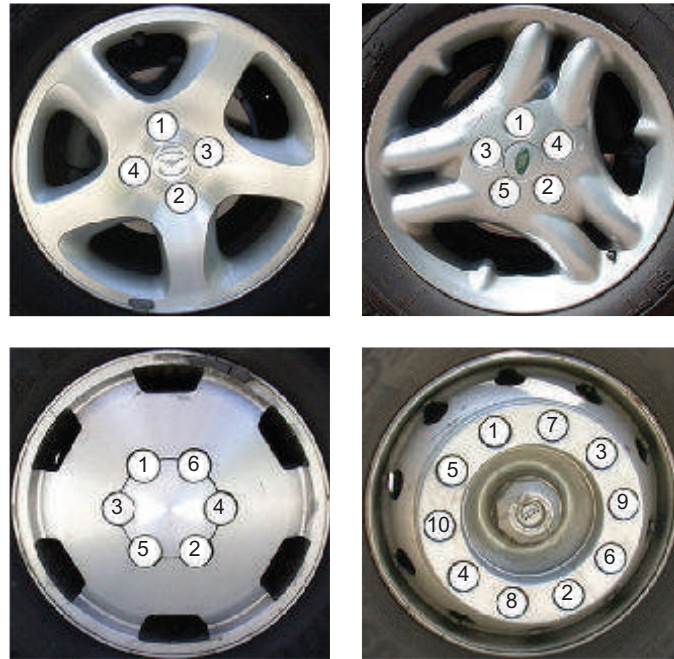
Figure 4.141 Torque sequences
