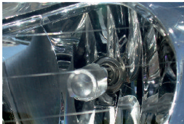
Figure 3.86 Headlights with a clear lens and complex reflector
