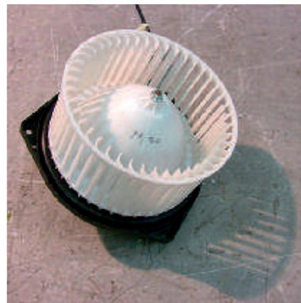
Figure 2.176 Heater motor fan
