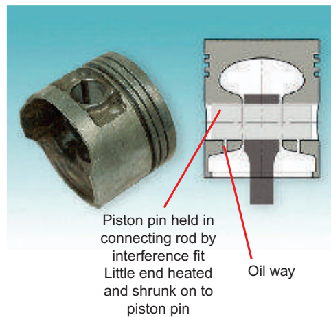
Figure 2.70 Piston pin in position
