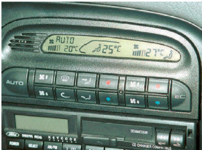
Figure 2.174 Air flow and heater controls
