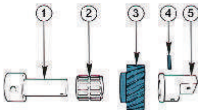
Figure 5.33 Reverse gear idler: 1, shaft; 2, needle roller bearing; 3, reverse gear idler; 4, roll pin; 5, mounting
