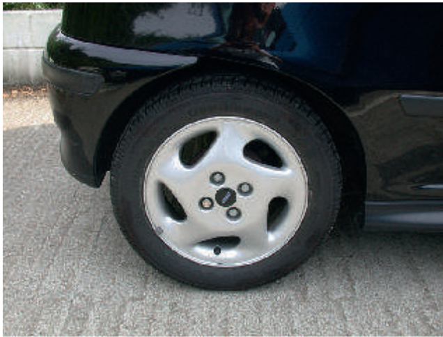
Figure 4.139 Four stud fixings
