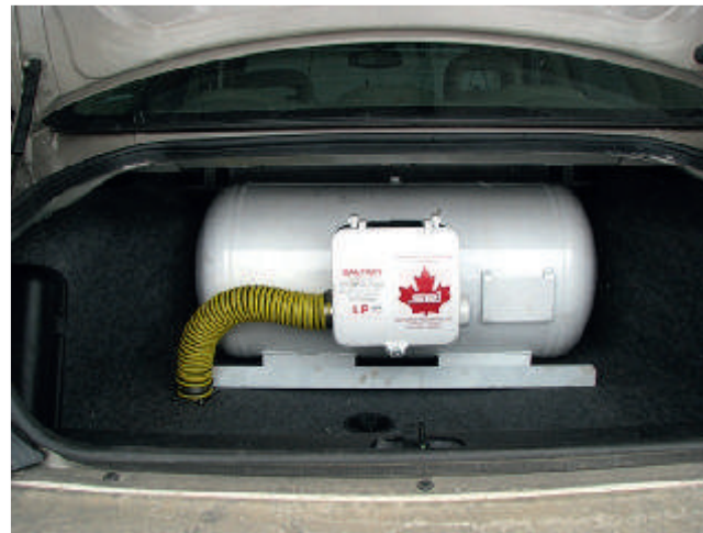
Figure 2.310 Propane tank. (Source: http://www.rasoenterprises.com )
