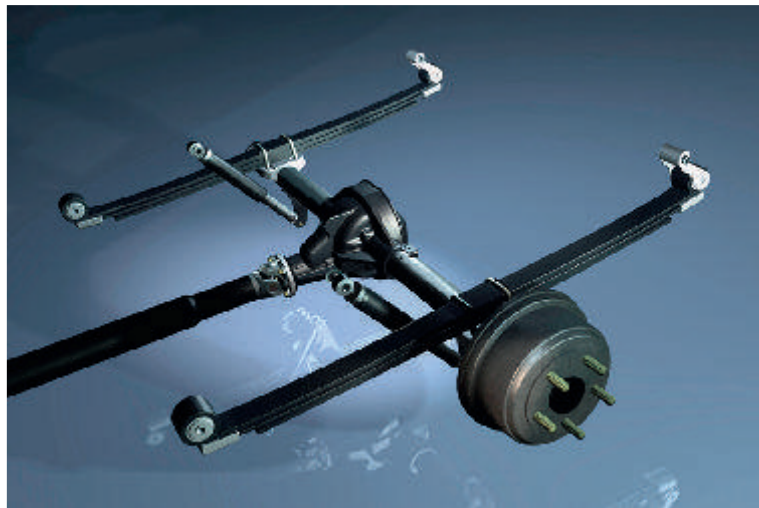
Figure 4.37 This method is used on older and larger vehicles with live, fixed rear axles
