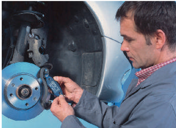
Figure 6.5 Fitting new brake pads. (Source: Bosch Media)
