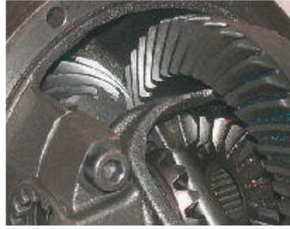
Figure 5.116 This differential is described as an open type
