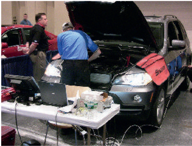
Figure 1.99 Bodywork protection in use during repairs
