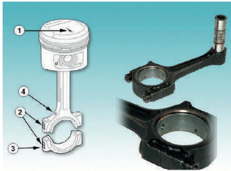
Figure 2.69 Con rod features: 1, front of engine; 2, identification marks; 3, big end cap; 4, oil spray hole for cylinder wall lubrication
