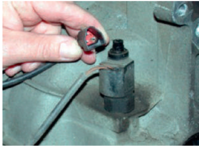
Figure 3.111 Road speed sensor in position
