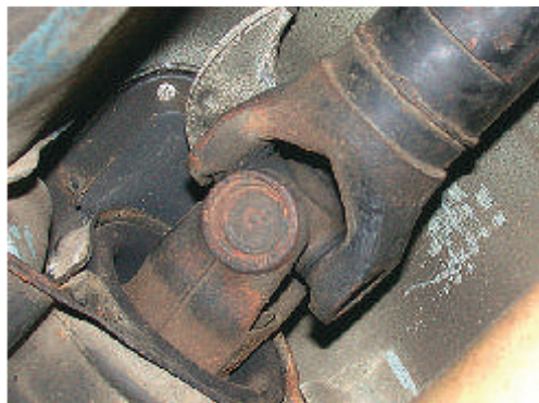
Figure 5.82 Universal joint in position
