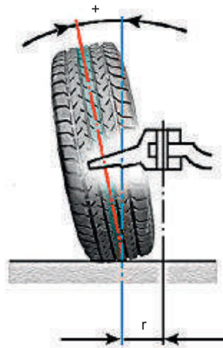
Figure 4.66 Positive camber ( r = scrub radius)
