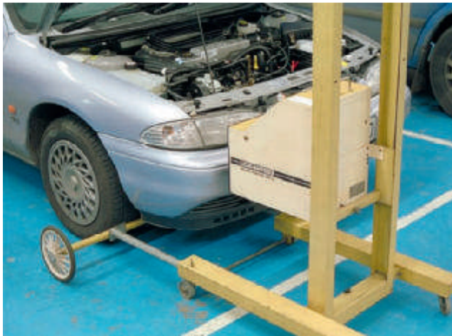
Figure 3.87 Beam setter in use
