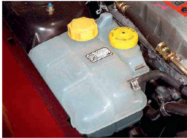
Figure 2.160 Remote expansion tank (on the left)
