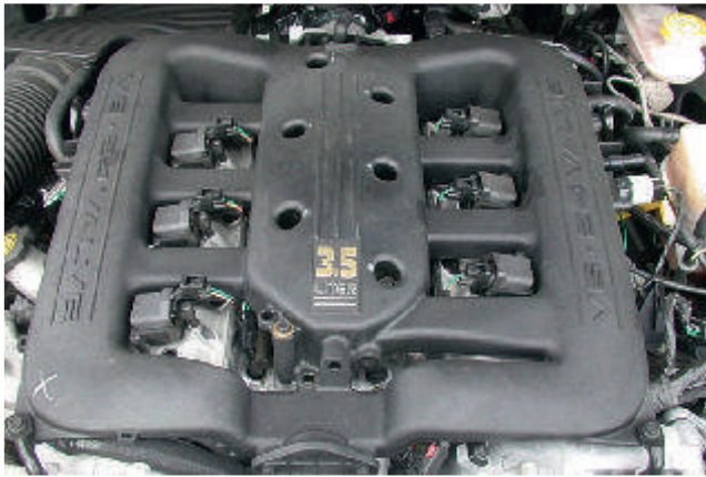
Figure 2.331 Six direct ignition coils in position
