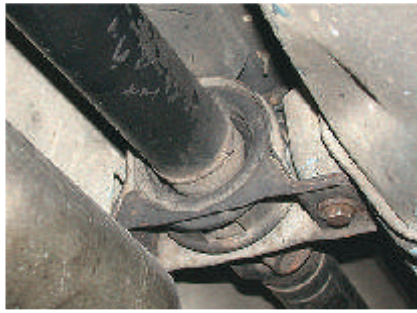
Figure 5.90 This rubber mounted bearing prevents propshaft whip
