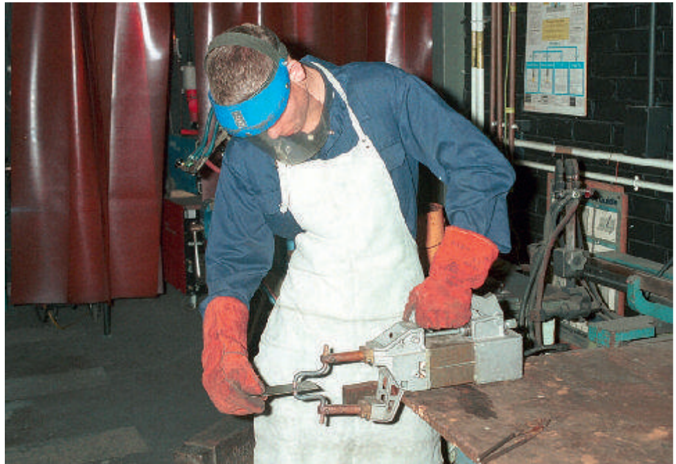
Figure 1.39 Protective clothing for spot welding
