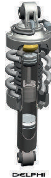
Figure 4.44 Suspension strut and actuator connection. (Source: Delphi Media)
