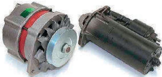
Figure 3.6 Reversibility: motor and generator
