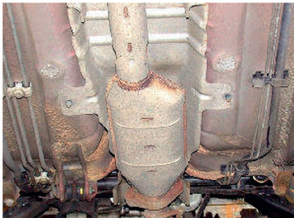
Figure 2.201 Catalytic converter in position with a heat shield above
