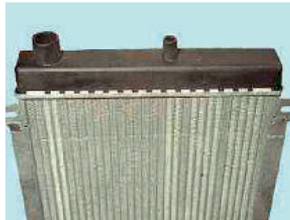
Figure 2.161 Aluminium and plastic radiator
