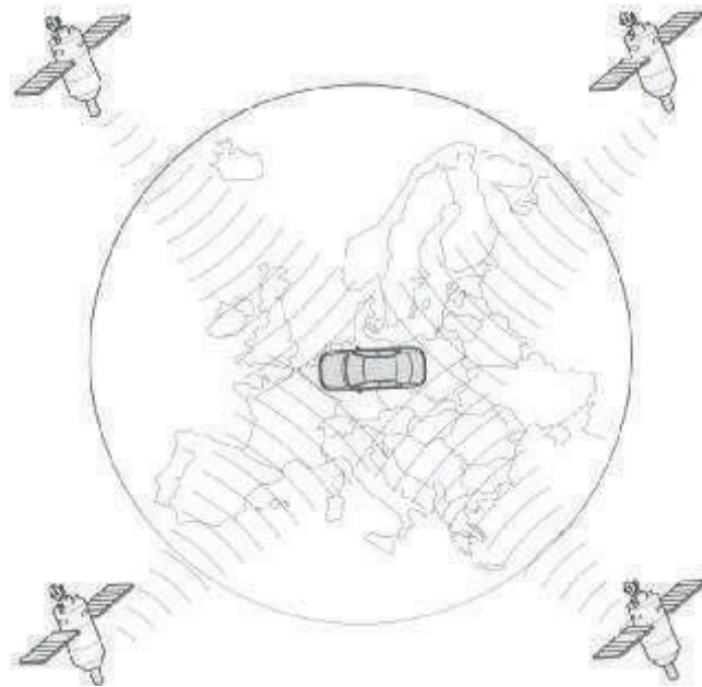
Figure 3.157 Four satellites determine vehicle position more accurately
