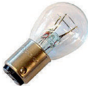
Figure 3.97 Stoplight and rear light twin filament bulb
