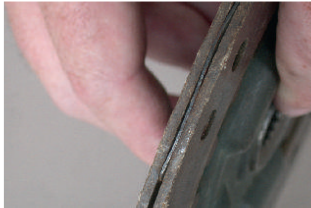
Figure 5.11 Wave springs eliminate chatter
